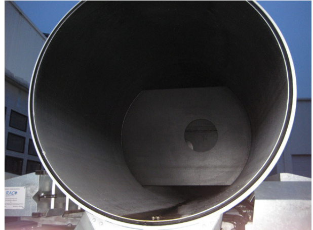
Inside view of vacuum tank
