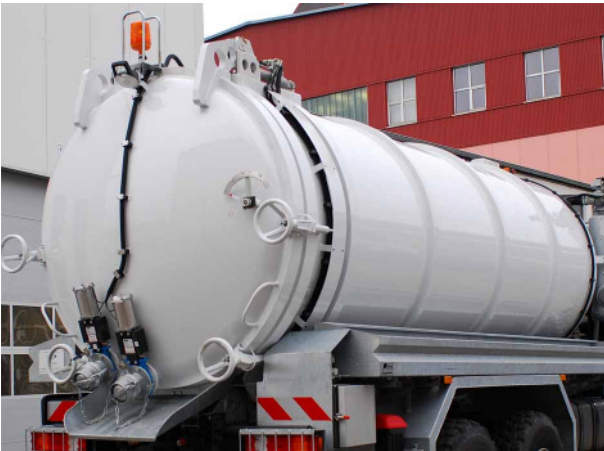
20.000 l. vacuum tank with top-mounted door
