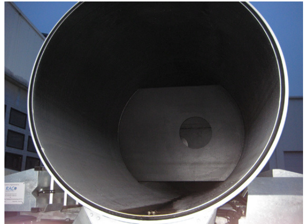
Inside view of vacuum tank
